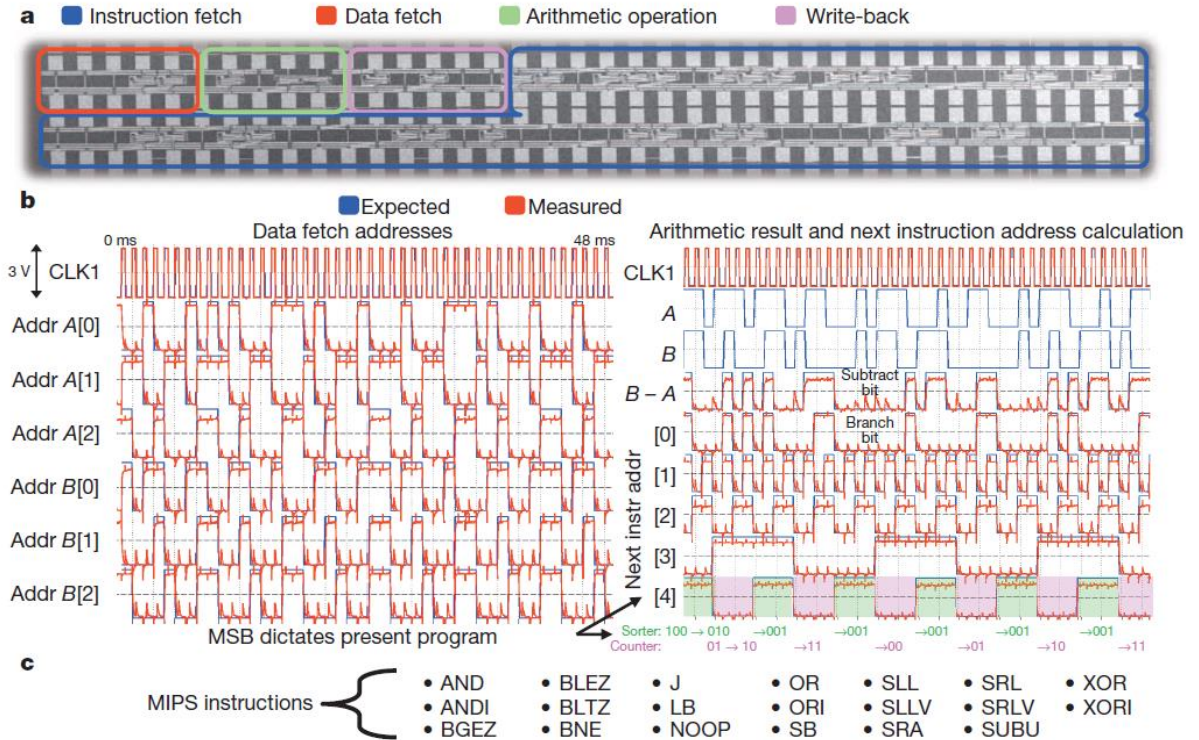
Figure 2.5. (a) SEM of an entire CNT computer. (b) Measured and expected output waveforms for a CNT computer, running the program of arithmetic unit. The exact match in logic value of the measured and expected output verifies correct operation. As shown by the most significant bit (MSB) (denoted [4]) of the next instruction address, the computer is switching between performing counting and sorting (bubble-sort algorithm). The running results of the counting and sorting are shown in the rows beneath the MSB of the next instruction address. (c), A list of the 20 MIPS instructions tested on the CNT computer. Reprinted with permission from [57]. Copyright (2013) Nature Publishing Group.
