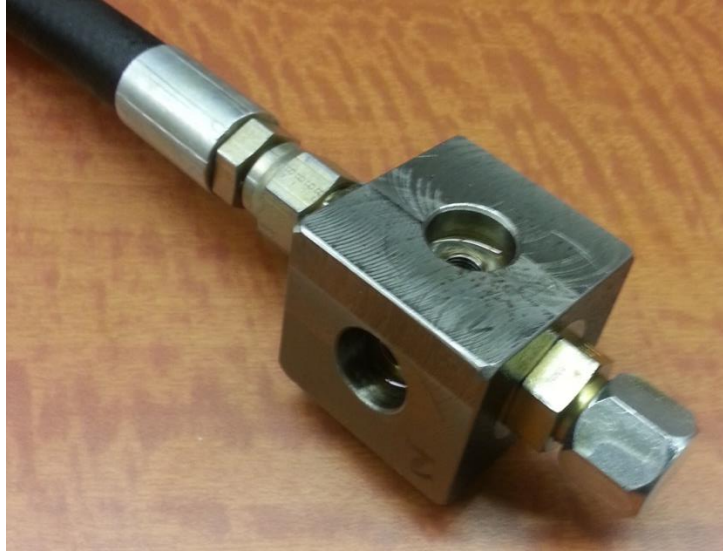
Figure 26: The calibration block without sensors
