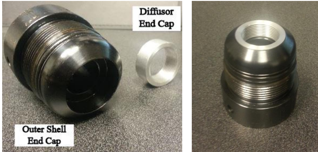
Figure 15: Mating between shell and diffuser end caps
