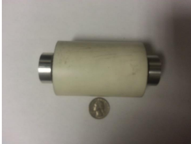
Figure 13: Fully assembled liner and diffuser combination
