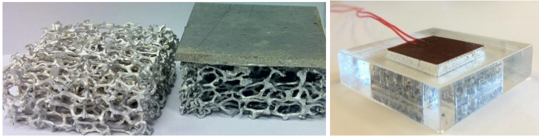
Figure 4.14 Aluminum foam before and after the attachment of the aluminum plate (left); Sample with heater attached to aluminum plate, foam saturated with PCM, and integrated into acrylic container (right).
