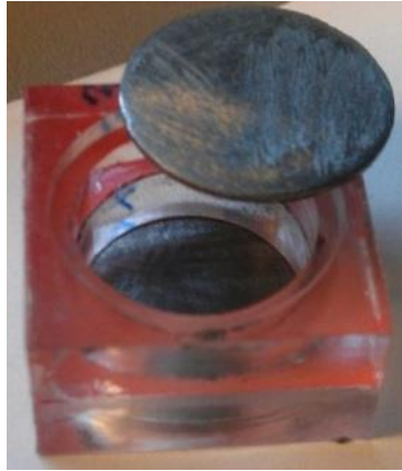
Figure 3.4 Test container for capacitance sedimentation measurements.
