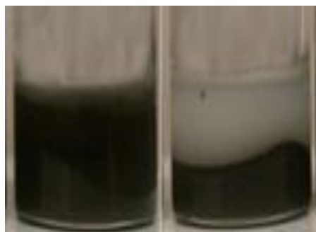
Figure 3.11 3 wt% xGnP-15, 50% paraffin/50% microcrystalline system (24 hour on left, 1 hour on right) after 2 hours in liquid state.
