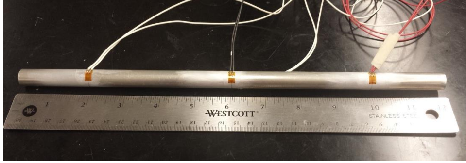
Figure 2.6 Aluminum validation sample with three strain gauges bonded in hoop direction and one strain gauge in an axial direction (away from the camera).
