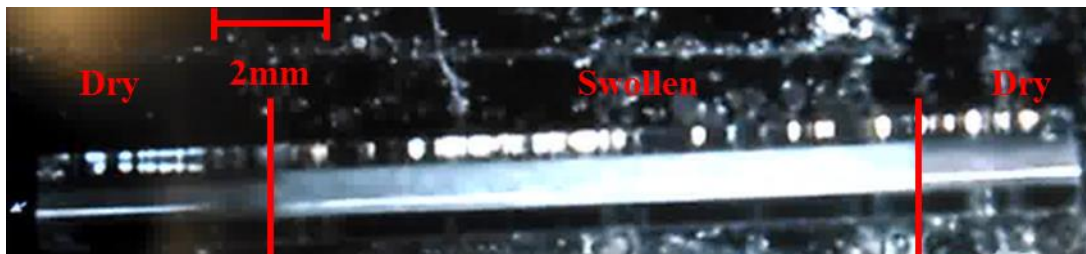
Figure 26: Evaporation of water within the hydrogel leads to regions dry polymer on the sample ends (opaque) while the middle length remains swollen (white).
