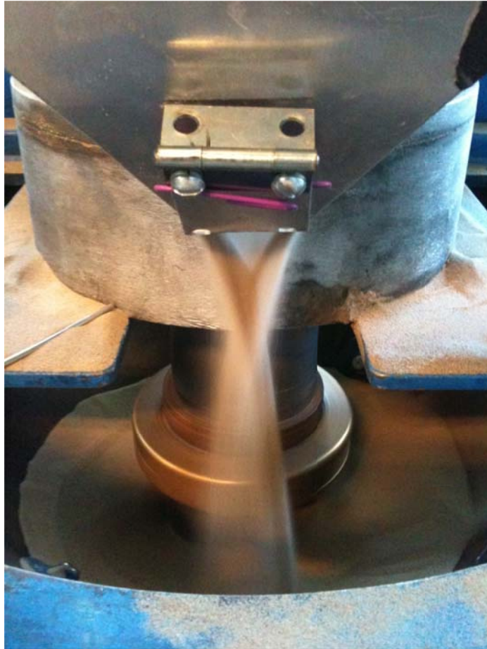
Figure 8: Chute to Consolidate Exit Flow
