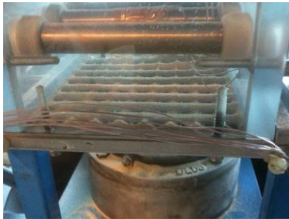
Figure 6: Particle Discharge Using a Cross-Hatched Pattern
