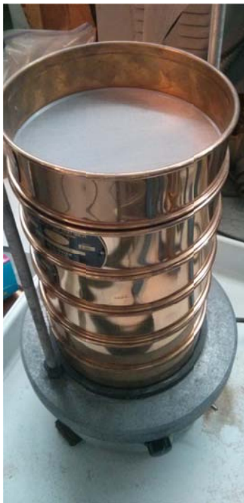
Figure 23: Sifting Device with Stacked Sieves
