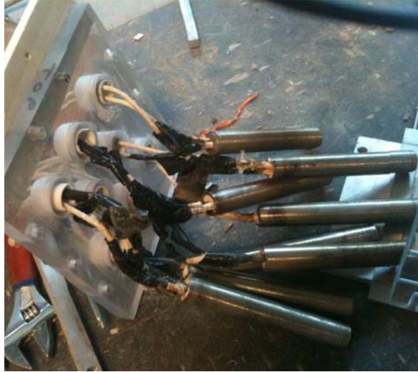
Figure 3: 8 Cartridge Heaters Held in Position by End Cap
