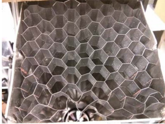
Figure 16: Honeycomb Structure to Provide Uniform Air
