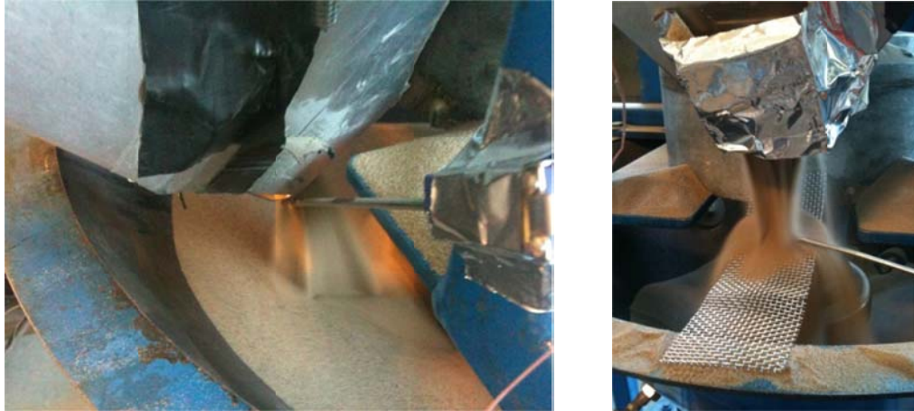
Figure 11: Attempts to Measure the Particulate Temperature
