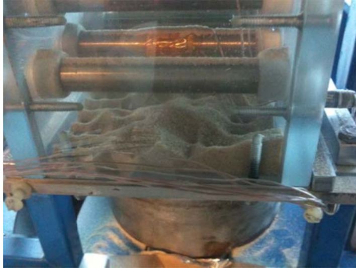
Figure 7: Evidence of Bridging Caused by Large Particulates
