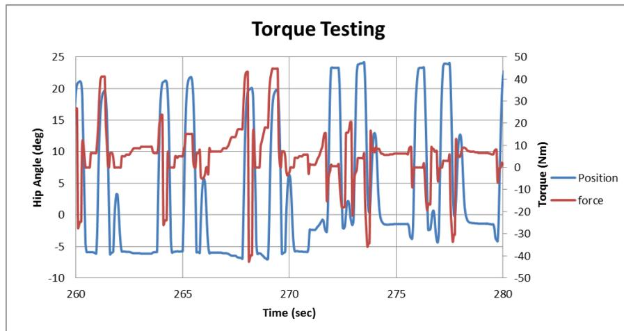
**Figure 6-11: Torque and position data when the user fights the exoskeleton and it provides its peak torque. For the 71 kg subject tested here, the exoskeleton must provide 44 Nm of torque and is successfully provided 44.6 Nm.**
