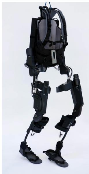
**Figure 2-2: Ekso exoskeleton**
