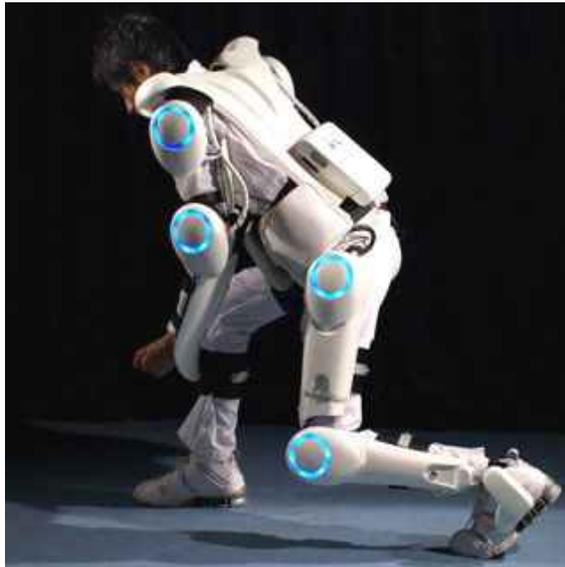
**Figure 2-1: HAL 5 exoskeleton**
