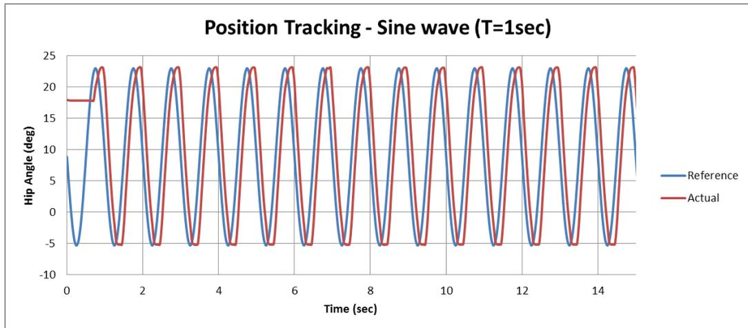
Figure 6-3: Position tracking of 1 Hz sine wave
