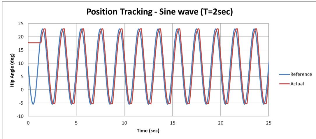
Figure 6-2: Position tracking of 0.5 Hz sine wave.
