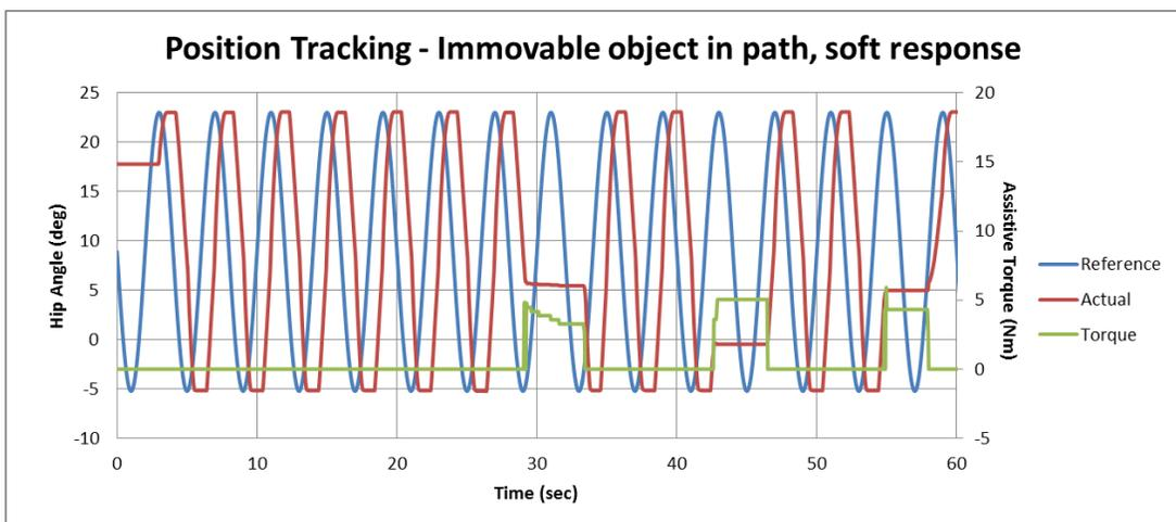
**Figure 6-7: Position tracking of a sine wave reference (4 second period) with a soft controller and an object put in the path of motion. The assistive torque is much lower than it was with the stiff controller.**
