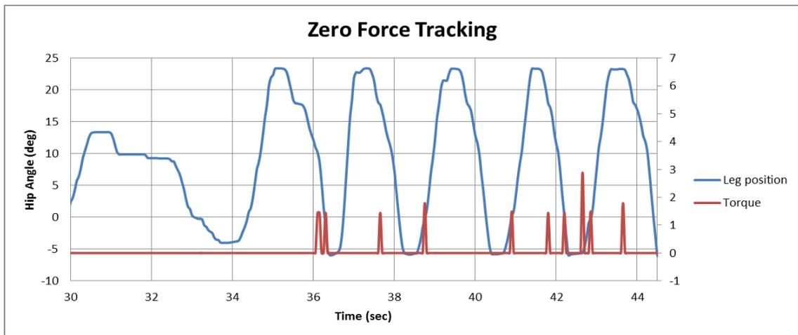
**Figure 6-8: The controller is in learning mode and works to minimize the interaction torque (Nm) between the exoskeleton and user. The leg bar was pushed back and forth by hand and the motor moved the yoke out of the way to reduce the force.**
