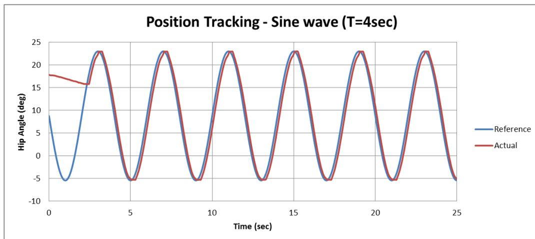
Figure 6-1: Position tracking of 0.25 Hz sine wave.
