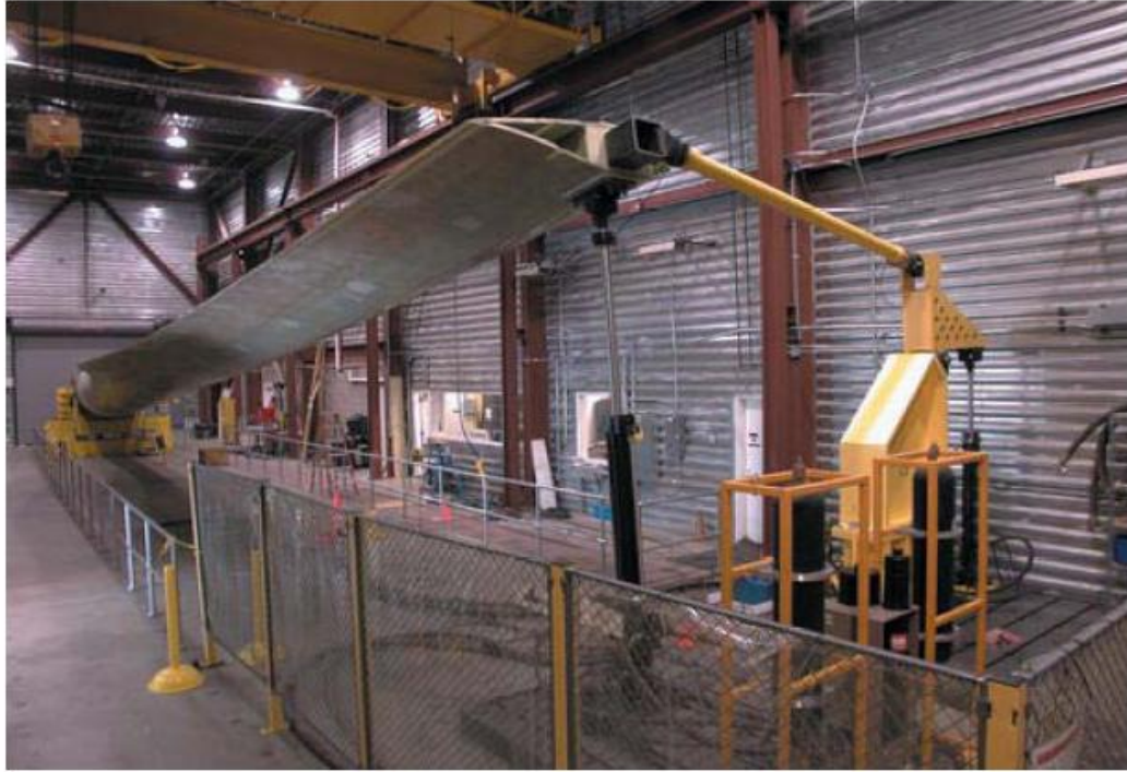
Figure 1.9 Dual-axis forced-displacement test system
