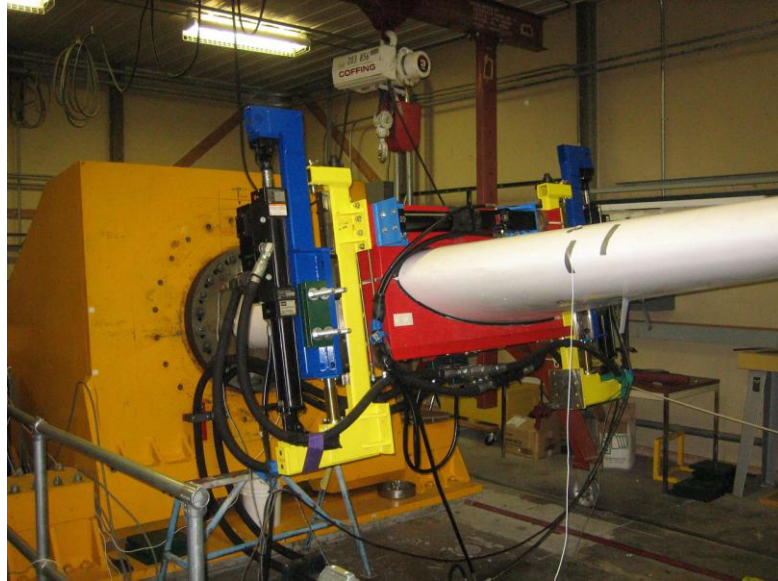
Figure 1.11 UREX dual axis resonance tests system (photo taken at NWTC, NREL)
