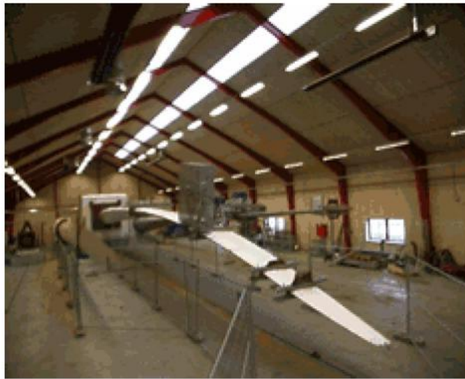
Figure 1.8 RISØ's single-axis resonance test system
