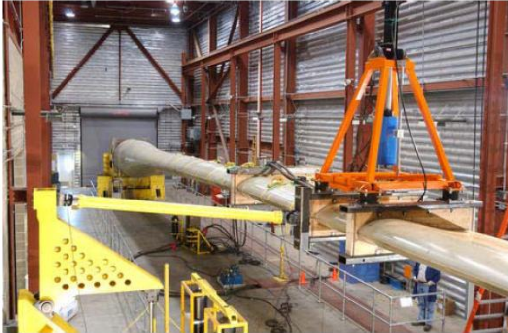
Figure 1.10 BREX dual axis resonance test system
