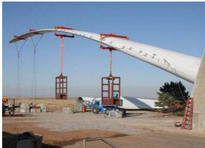
Figure 1.7 Static Testing using ballast weights and winches
