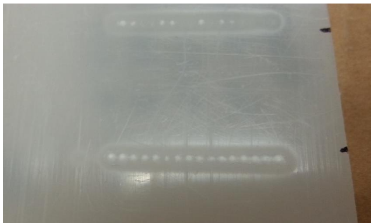
Figure 2-13. Photo of 'dots' of deposition resulting from discontinuous powder feed. Sample is BYK Ceraflour 916 sprayed onto LDPE substrate at 25°C and 50 psi.
