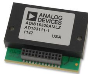
Figure 6-5. Four degrees of freedom inertial sensor (ADIS16300).
