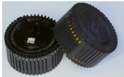
Figure 6-4. Puck™ (B3880) servo electronics module from Barrett Technology.
