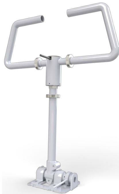
Figure 8-2. Handlebar assembly of the TWIP prototype.
