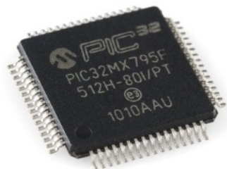
Figure 6-2. 32-bit PIC microcontroller (PIC32MX795F512H).
