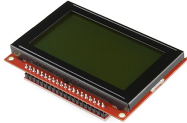
Figure 6-6. Serial graphic LCD 128x64 (LCD-09351).
