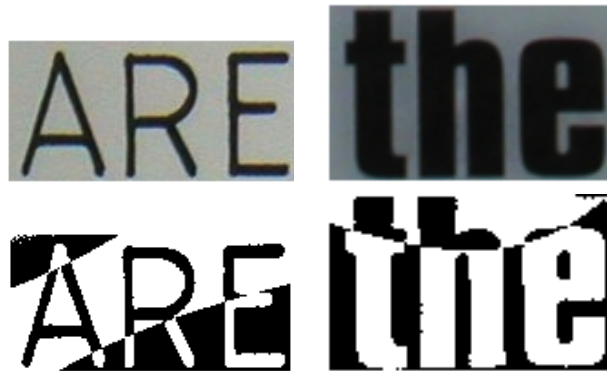
Figure 6.3: Sample segmentations that result from poor initialization using a mixture of two regressions.
