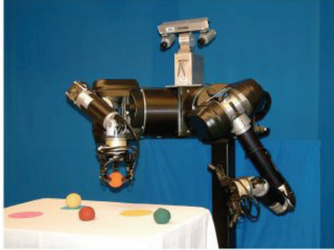
Figure 3.6. Dexter is a bimanual upper-body humanoid.
