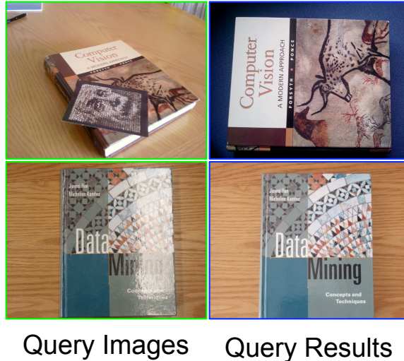
Figure 5.4. Examples of book cover search results. The first column shows queries and the top results are shown in the second column. The technique is resilient to occlusions and viewpoint change (top left image) and specularities (bottom left image).
