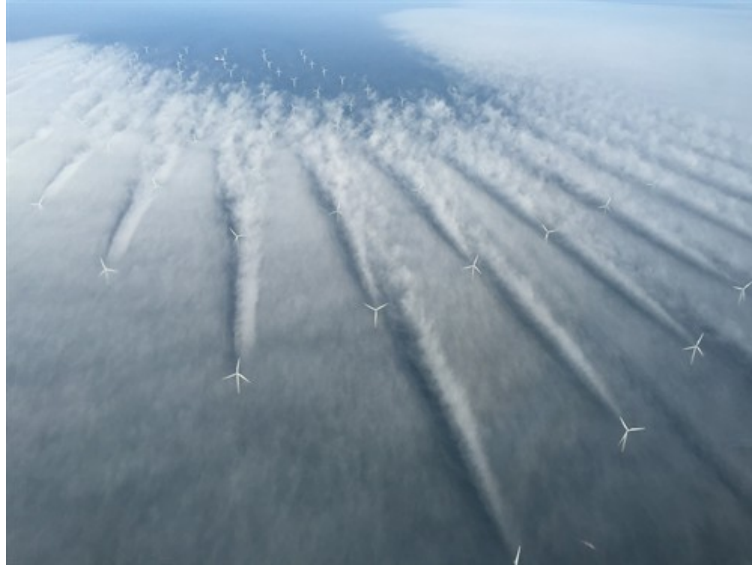
Figure 2.11: Wake merging in the Horns Rev wind farm [4].
