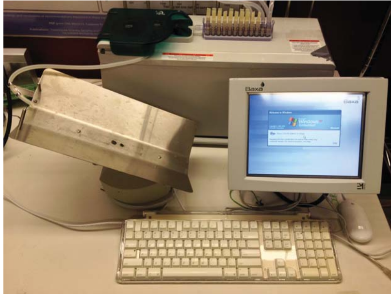
Figure 5.2: Running on Windows XP Embedded SP2, our Baxa ExactaMix 2400 pharmaceutical compounder is an automated embedded system that mixes liquids to individual specifications for intravenous parenteral nutrition.
