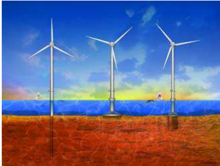
Figure 2.6. Three shallow water wind turbine foundations; the monopile, the gravity base, and the suction bucket from right to left [31].
