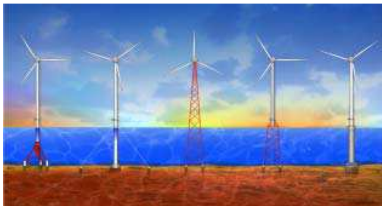
Figure 2.7. Transitional water depth foundation designs. [31].
