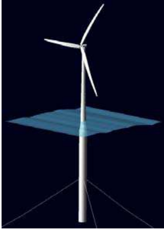
Figure 2.12. Graphic depicting the OC3-Hywind Spar Buoy
