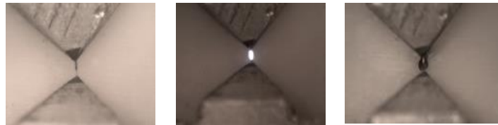
Figure. 1.2. Electrode life time, Pd Electrodes (50 µm diameter) N 2 Gas, 1 mA (~0.5 W) steady state for 10(+) minutes, (Courtesy Dr. David Staack Texas A&M University).
