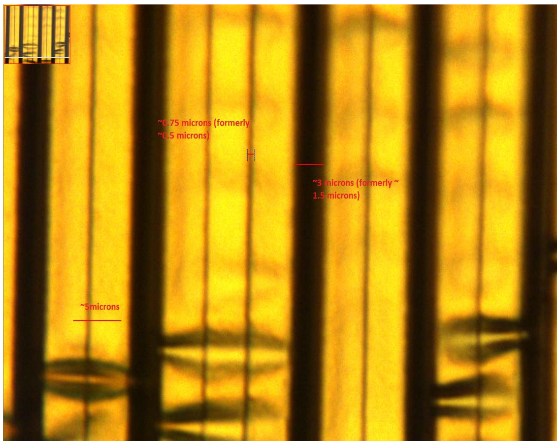
Figure 24: Crack Test Results Gold-Coated sample under maximum strain. No crack formation is immediately visible ( 5 \mu\text{m} scale in lower left)
