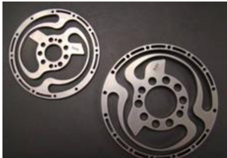
Figure 2.9 Springs used in Robonaut 2's SEAs [15]
