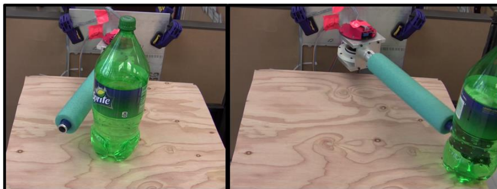
Figure 6.5 The SEA prototype with an object obstructing its trajectory (left) and after the object has been moved when using high impedance (right)
