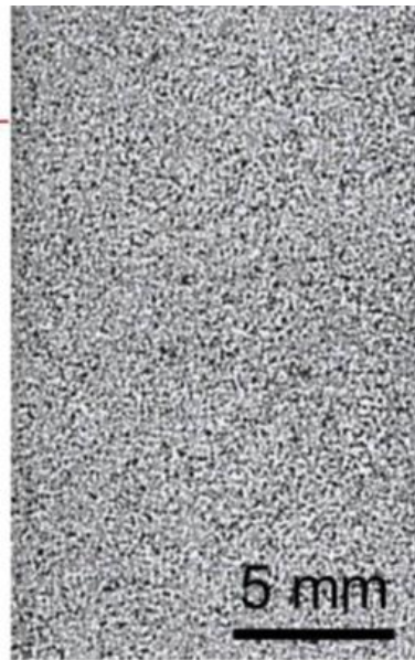
Figure 2.13. Typical high temperature resistant speckle pattern used
