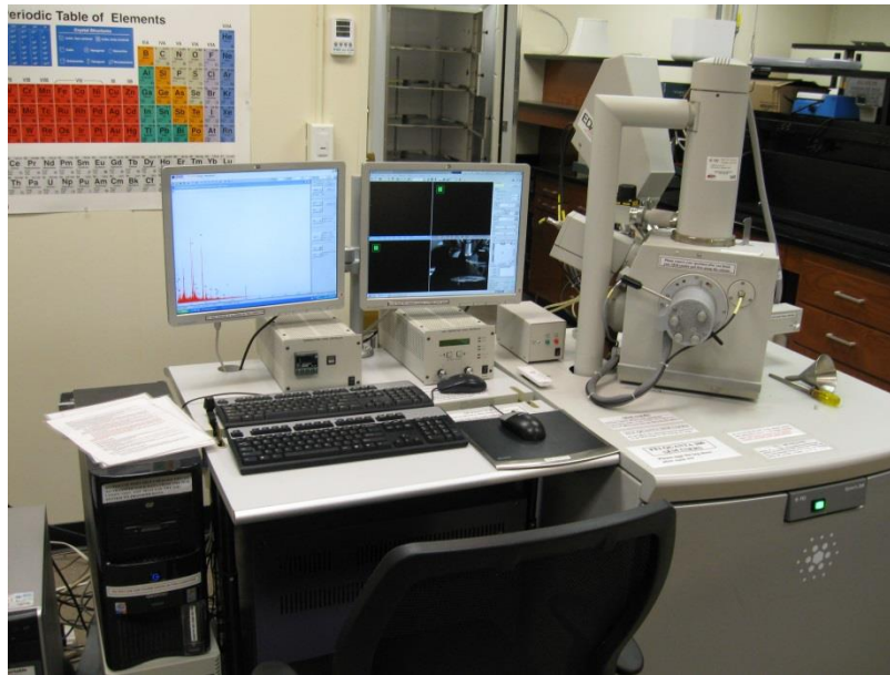
Figure 2.25 Quanta 200 Environmental Scanning Electron Microscope (ESEM)
