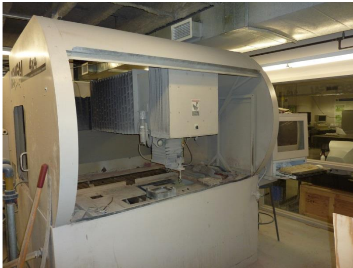
Figure 2.16 Bengal water jet cutting machine
