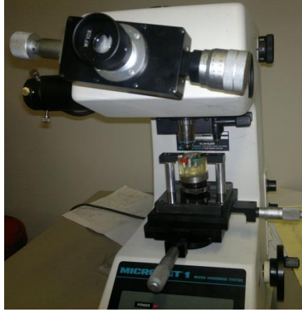
Figure 2.20 Buehler Micromet 1 hardness test machine
