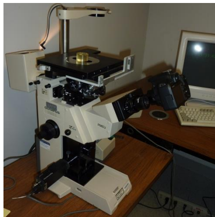
Figure 2.18 Leo Olympus PME3 inverted metallurgical microscope
