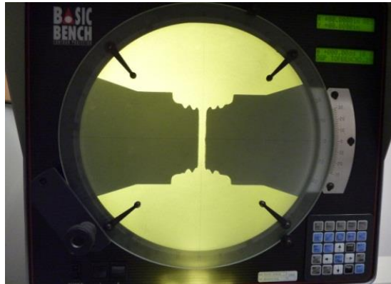
Figure 2.4 Comparison between LH&RH threaded pin by BASIC BENCH contour projector
