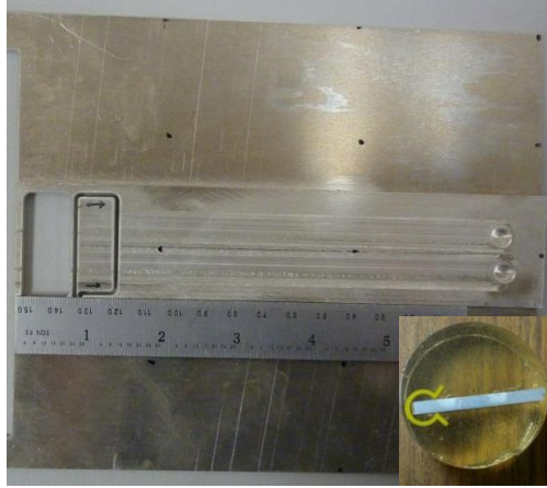
Figure 2.17 Sample cut from weldment and sample placed in the epoxy
