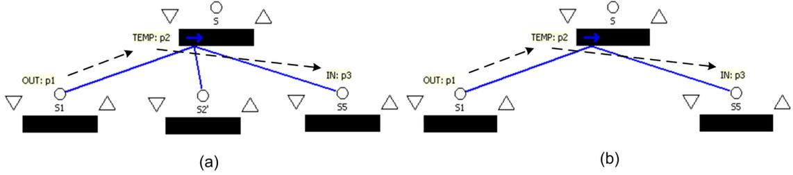
**Figure 4.11.** Step Removal for Fault Tree Derivation
