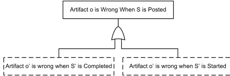
**Figure 4.7.** Partial Fault Tree for Template 2
