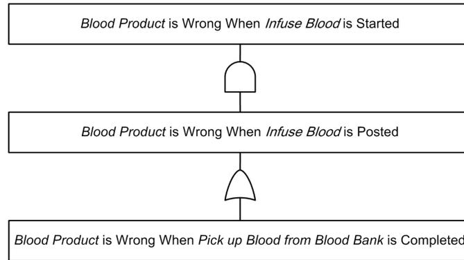
**Figure 4.8.** Instantiated Partial Fault Tree for Template 2
