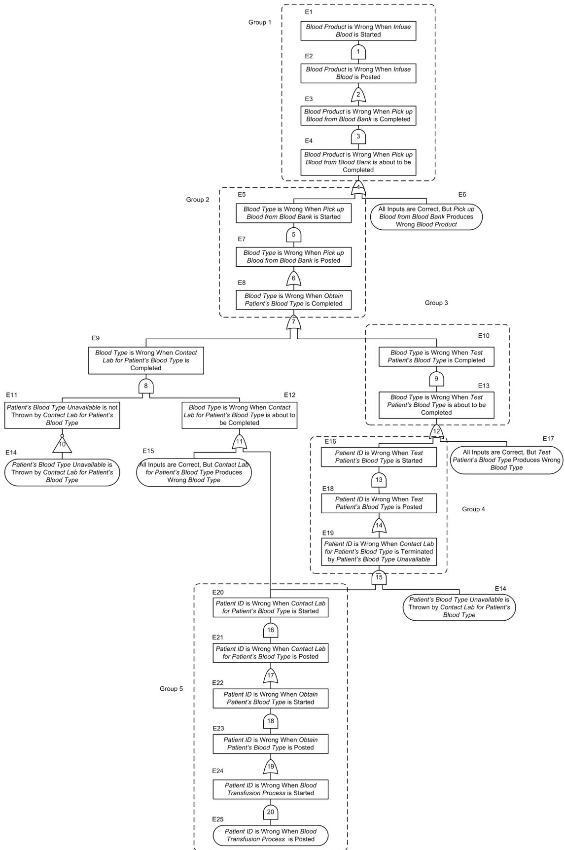
Figure 4.12. Groups in Fault Tree for Simplified Blood Transfusion Process
