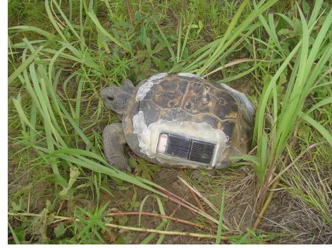
Figure 3.2. A gopher tortoise equipped with a TurtleNet tracking device.
