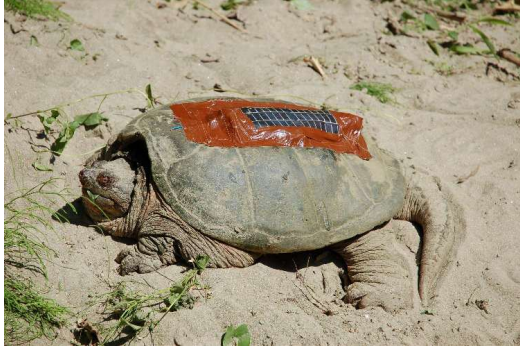
Figure 3.1. An early TurtleNet test deployment on a snapping turtle.
