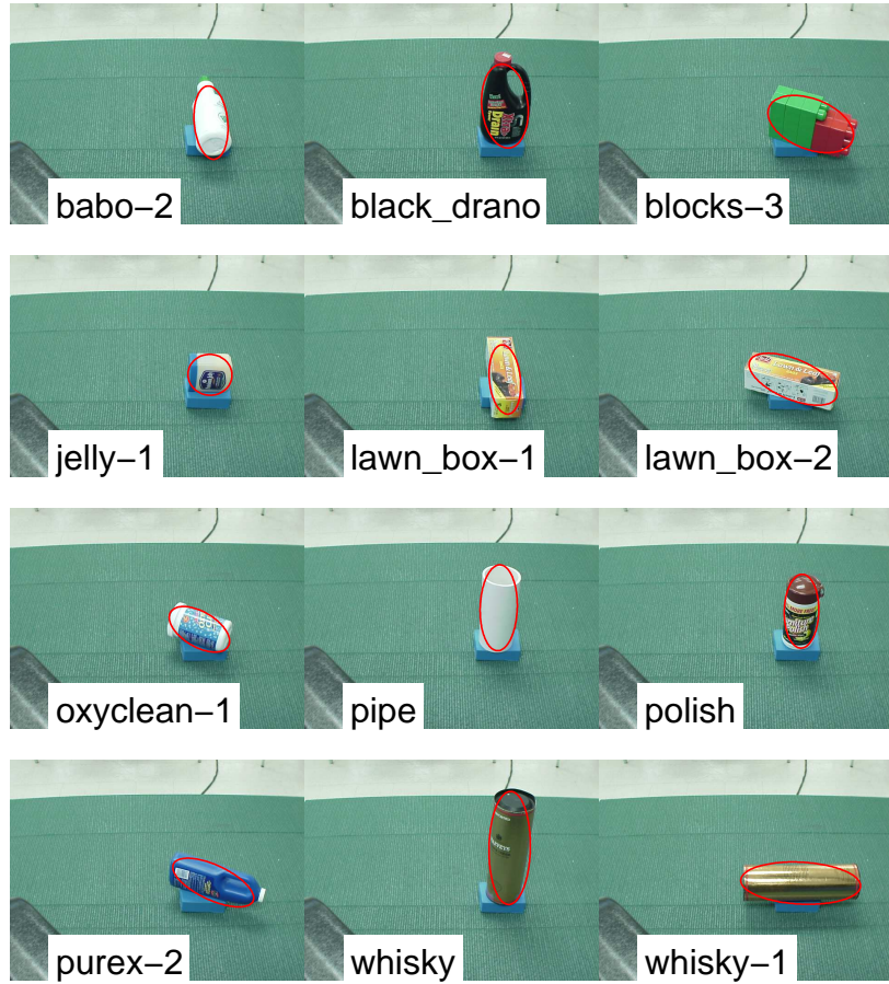
Figure 6.5. This picture shows the objects as they were presented for generating grasps. The red oval corresponds to the covariance matrix that was computed from the average second moments of the segmented blob in the left and right cameras.
