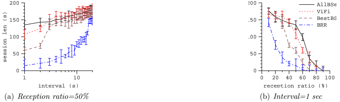
Figure 5.6. ViFi: The median session length in VanLAN as a function of the reception ratio threshold and time interval used to define adequate connectivity.
