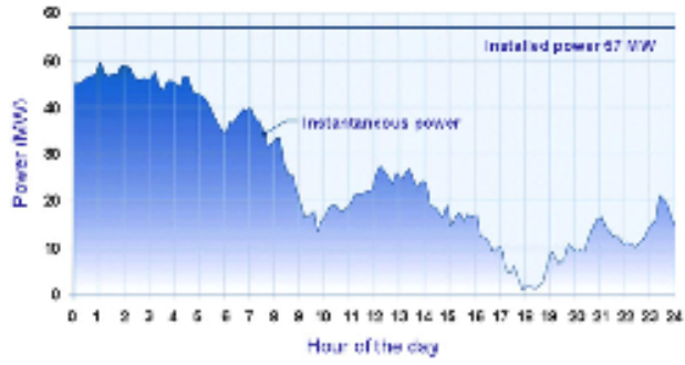
Figure9: Power generation on March 16, 2004 at Cap-Chat wind farm (Canada) [16]
