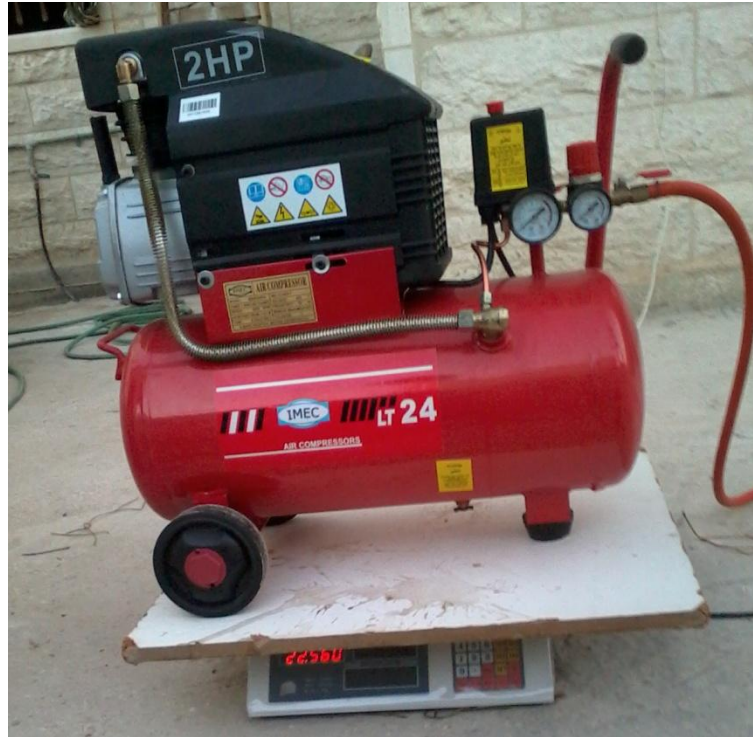
Figure 5: Weighing the compressor using the electronic balance
