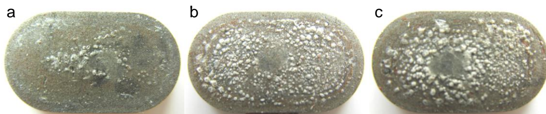
Figure 3.5: Particulate deposited on porous media following continual use in combustion chamber (a – c). These fluidic valves are identical in size with valves in Figure 3.4c & d.
