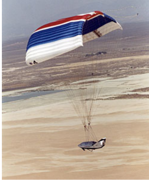
Figure 1.3: NASA X38 with 7,500 ft 2 canopy deployed [16].
