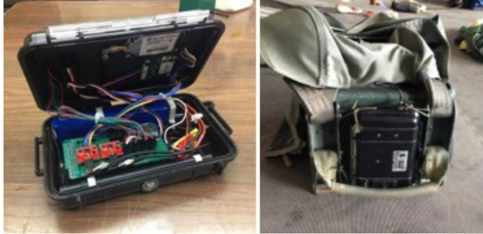
Figure 6.10: Payload relay box internal components (left) and mounted on MC-4/5 AGU (right) prior to test flight.
