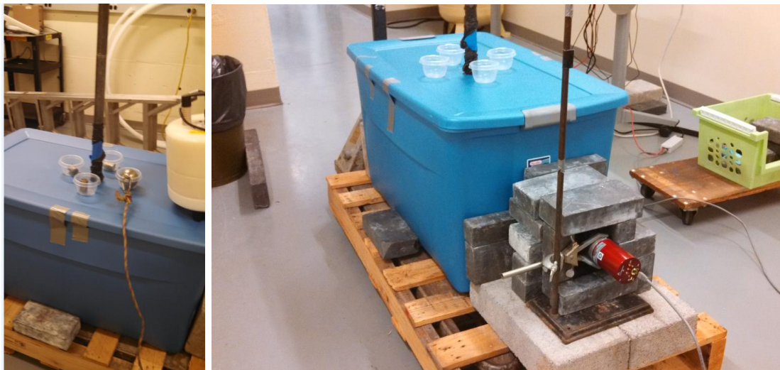
Figure 3.18: Actual experimental setup. Left: Sources in place. Right: Detector with Pb sheilding.
