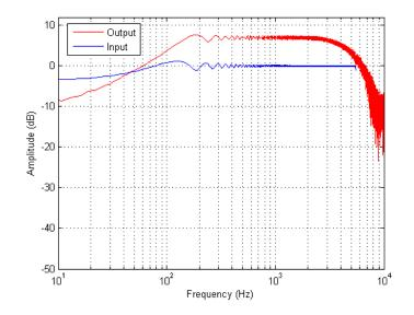
Figure 121. Haptic Board Voltage Output Frequency Plots – Sine Sweep, 12 dB gain, 35 Volume, No-load Impedance Condition
