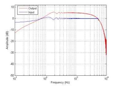
Figure 136. Frequency Spectrum –Haptic Board Voltage Measurement – No load – Sine Sweep, 6 dB Gain, 35 Volume
