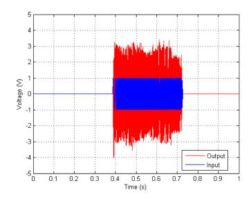
Figure 137. Time Spectrum –Haptic Board Voltage Measurement – No load – Sine Sweep, 6 dB Gain, 36 Volume
