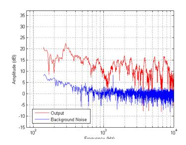
Figure 234. Audio Frequency Spectrum – Pack 9 Switch 3
