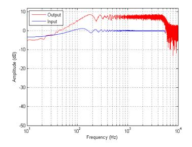
Figure 125. Haptic Board Voltage Output Frequency Plots – Sine Sweep, 24 dB gain, 35 Volume, No-load Impedance Condition
