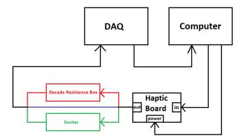
Figure 7: Haptic Board Voltage Output Experimental Setup. No-Load Setup in Blue, Exciter Loaded Setup in Green, Resistor Loaded Setup in Red.
