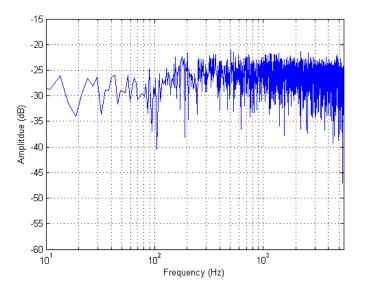
Figure 17. Haptic Board Voltage Output Transfer Functions – Sine Sweep, 6 dB gain, 36 Volume, No-load Impedance Condition
