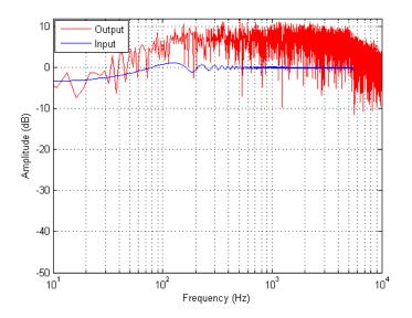
Figure 126. Haptic Board Voltage Output Frequency Plots – Sine Sweep, 24 dB gain, 36 Volume, No-load Impedance Condition
