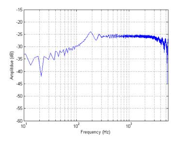
Figure 14. Haptic Board Voltage Output Transfer Functions – Sine Sweep, 6 dB gain, 35 Volume, No-load Impedance Condition
