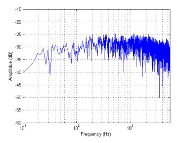
Figure 25. Haptic Board Voltage Output Transfer Functions – Sine Sweep, 6 dB gain, 36 Volume, No-load Impedance Condition
