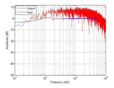
Figure 122. Haptic Board Voltage Output Frequency Plots – Sine Sweep, 12 dB gain, 36 Volume, No-load Impedance Condition
