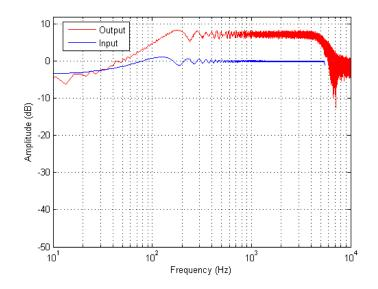
Figure 123. Haptic Board Voltage Output Frequency Plots – Sine Sweep, 18 dB gain, 35 Volume, No-load Impedance Condition
