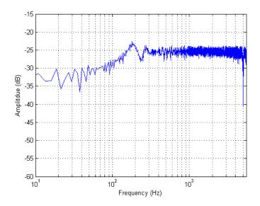
Figure 16. Haptic Board Voltage Output Transfer Functions – Sine Sweep, 6 dB gain, 35 Volume, No-load Impedance Condition
