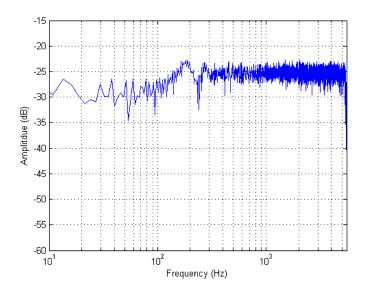
Figure 18. Haptic Board Voltage Output Transfer Functions – Sine Sweep, 24 dB gain, 35 Volume, No-load Impedance Condition
