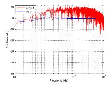
Figure 124. Haptic Board Voltage Output Frequency Plots – Sine Sweep, 18 dB gain, 36 Volume, No-load Impedance Condition
