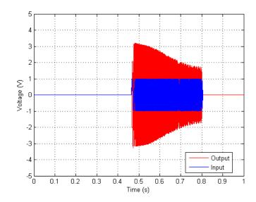
Figure 131. Time Spectrum –Haptic Board Voltage Measurement – Resistor loaded – Sine Sweep, 6 dB Gain, 35 Volume
