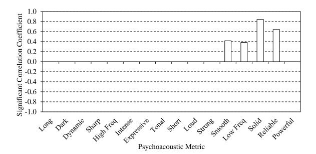
Figure 66. Significant Correlation Coefficient vs. Psychoacoustic Metric: Volume Down-. Parametric Metrics Used the Pearson Product Moment Correlation Coefficient. Non-Parametric Metrics Used Spearman's Rank-Order Correlation Coefficient.
