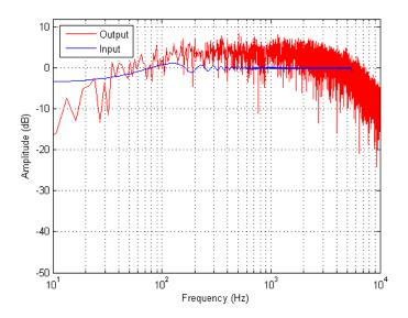
Figure 130. Frequency Spectrum –Haptic Board Voltage Measurement – Exciter loaded – Sine Sweep, 6 dB Gain, 36 Volume
