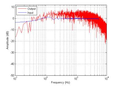
Figure 120. Haptic Board Voltage Output Frequency Plots – Sine Sweep, 6 dB gain, 36 Volume, No-load Impedance Condition
