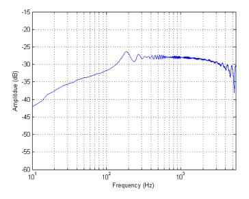
Figure 20. Haptic Board Voltage Output Transfer Functions – Sine Sweep, 6 dB gain, 35 Volume, Exciter loaded Impendence Condition
