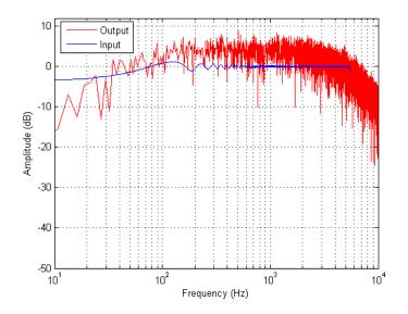
Figure 138. Frequency Spectrum –Haptic Board Voltage Measurement – No load – Sine Sweep, 6 dB Gain, 36 Volume
