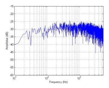
Figure 21. Haptic Board Voltage Output Transfer Functions – Sine Sweep, 6 dB gain, 36 Volume, Exciter loaded Impendence Condition
