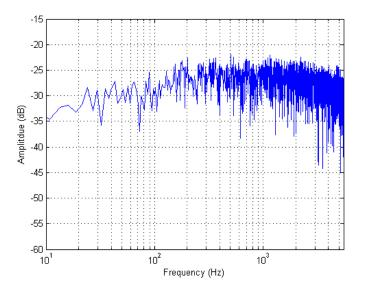
Figure 15. Haptic Board Voltage Output Transfer Functions – Sine Sweep, 6 dB gain, 36 Volume, No-load Impedance Condition
