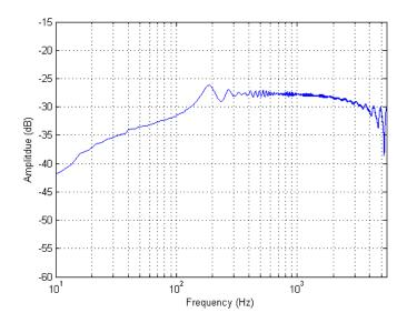
Figure 24. Haptic Board Voltage Output Transfer Functions – Sine Sweep, 6 dB gain, 35 Volume, No-load Impedance Condition
