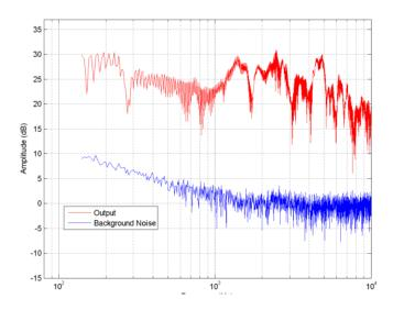
Figure 204. Audio Frequency Spectrum – Pack 6 Switch 4
