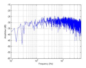
Figure 23. Haptic Board Voltage Output Transfer Functions – Sine Sweep, 6 dB gain, 36 Volume, Resistor loaded Impendence Condition
