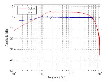
Figure 132. Frequency Spectrum –Haptic Board Voltage Measurement – Resistor loaded – Sine Sweep, 6 dB Gain, 35 Volume
