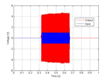
Figure 115. Haptic Board Voltage Output Time Plots – Sine Sweep, 18 dB gain, 35 Volume, No-load Impedance Condition
