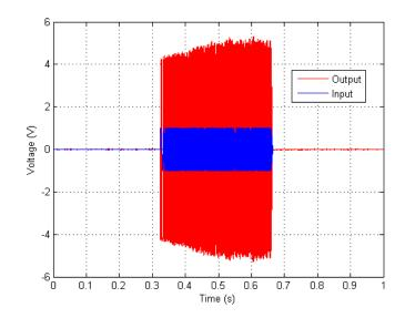
Figure 117. Haptic Board Voltage Output Time Plots – Sine Sweep, 24 dB gain, 35 Volume, No-load Impedance Condition
