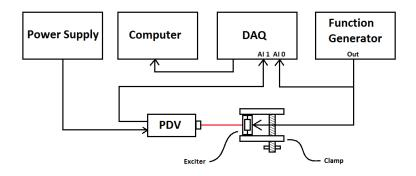
Figure 8: Exciter Output Experimental Setup
