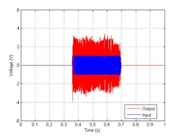
Figure 112. Haptic Board Voltage Output Time Plots – Sine Sweep, 6 dB gain, 36 Volume, No-load Impedance Condition
