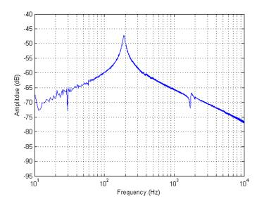
Figure 26. Exciter Transfer Function
