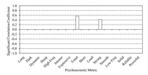
Figure 55. Significant Correlation Coefficient vs. Psychoacoustic Metric: On–. Parametric Metrics Used the Pearson Product Moment Correlation Coefficient. Non-Parametric Metrics Used Spearman's Rank-Order Correlation Coefficient.
