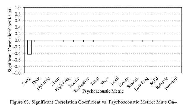
Figure 63. Significant Correlation Coefficient vs. Psychoacoustic Metric: Mute On–. Parametric Metrics Used the Pearson Product Moment Correlation Coefficient. Non-Parametric Metrics Used Spearman's Rank-Order Correlation Coefficient.
