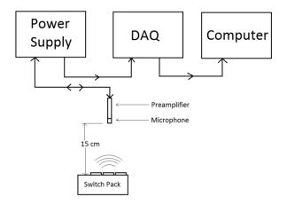
Figure 5. Switch Pack Audio Experimental Setup
