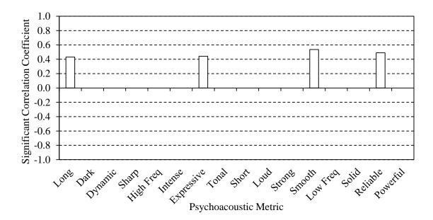
Figure 60. Significant Correlation Coefficient vs. Psychoacoustic Metric: Next Track–. Parametric Metrics Used the Pearson Product Moment Correlation Coefficient. Non-Parametric Metrics Used Spearman's Rank-Order Correlation Coefficient.
