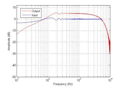
Figure 119. Haptic Board Voltage Output Frequency Plots – Sine Sweep, 6 dB gain, 35 Volume, No-load Impedance Condition
