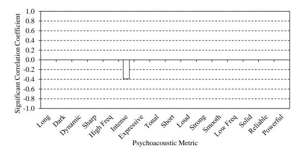
Figure 59. Significant Correlation Coefficient vs. Psychoacoustic Metric: Media Mode–. Parametric Metrics Used the Pearson Product Moment Correlation Coefficient. Non-Parametric Metrics Used Spearman's Rank-Order Correlation Coefficient.
