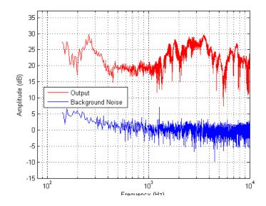
Figure 156. Audio Frequency Spectrum – Pack 2 Switch 1
