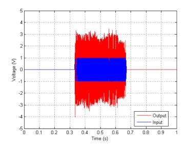
Figure 133. Time Spectrum –Haptic Board Voltage Measurement – Resistor loaded – Sine Sweep, 6 dB Gain, 36 Volume
