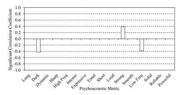
Figure 65. Significant Correlation Coefficient vs. Psychoacoustic Metric: Volume Up–. Parametric Metrics Used the Pearson Product Moment Correlation Coefficient. Non-Parametric Metrics Used Spearman's Rank-Order Correlation Coefficient.
