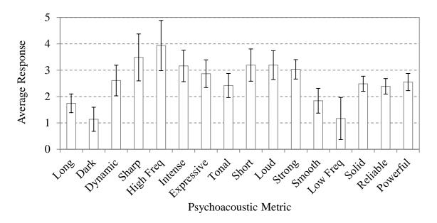
Figure 32. Response vs. Psychoacoustic Metric: Sample 6. The Response Scale Ranges From 1 = Not At All to 5 = Extremely.
