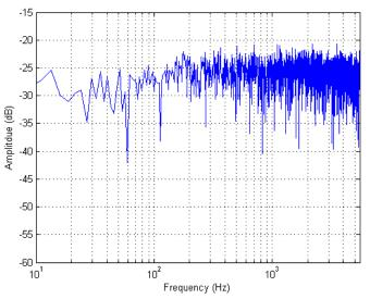
Figure 19. Haptic Board Voltage Output Transfer Functions – Sine Sweep, 24 dB gain, 36 Volume, No-load Impedance Condition
