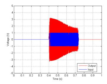
Figure 135. Time Spectrum –Haptic Board Voltage Measurement – No load – Sine Sweep, 6 dB Gain, 35 Volume
