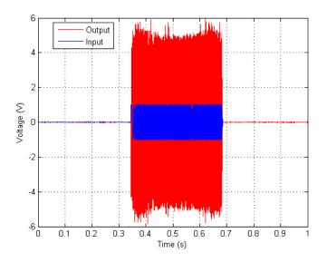
Figure 118. Haptic Board Voltage Output Time Plots – Sine Sweep, 24 dB gain, 36 Volume No-load Impedance Condition
