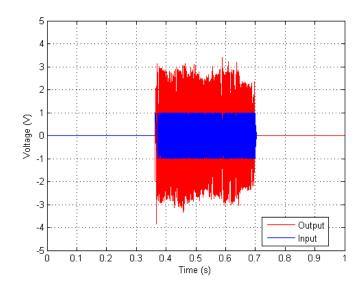
Figure 129. Time Spectrum –Haptic Board Voltage Measurement – Exciter loaded – Sine Sweep, 6 dB Gain, 36 Volume
