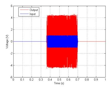
Figure 114. Haptic Board Voltage Output Time Plots – Sine Sweep, 12 dB gain, 36 Volume, No-load Impedance Condition
