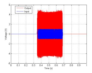
Figure 116. Haptic Board Voltage Output Time Plots – Sine Sweep, 18 dB gain, 36 Volume, No-load Impedance Condition
