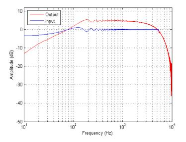
Figure 128. Frequency Spectrum –Haptic Board Voltage Measurement – Exciter loaded – Sine Sweep, 6 dB Gain, 35 Volume
