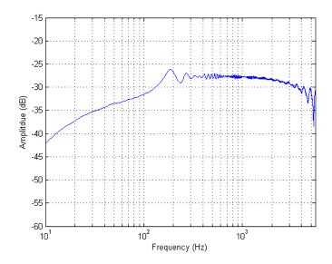
Figure 22. Haptic Board Voltage Output Transfer Functions – Sine Sweep, 6 dB gain, 35 Volume, Resistor loaded Impendence Condition
