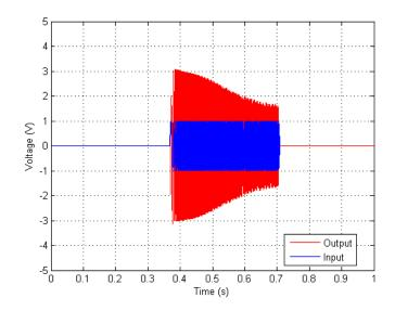
Figure 127. Time Spectrum –Haptic Board Voltage Measurement – Exciter loaded – Sine Sweep, 6 dB Gain, 35 Volume
