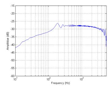
Figure 12. Haptic Board Voltage Output Transfer Functions – Sine Sweep, 6 dB gain, 35 Volume, No-load Impedance Condition
