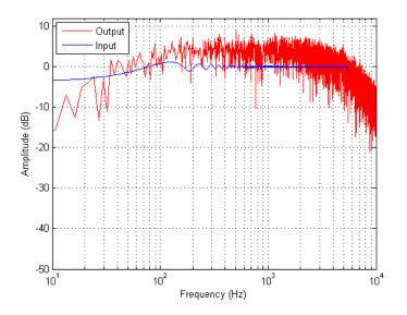
Figure 134. Frequency Spectrum –Haptic Board Voltage Measurement – Resistor loaded – Sine Sweep, 6 dB Gain, 36 Volume
