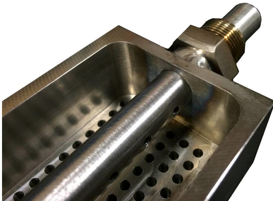
Figure 3.23 Close-up photograph of header and distributor before assembly
