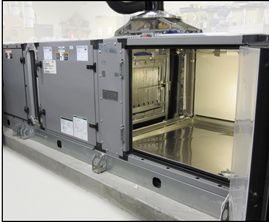
Figure 4.8 Photograph of absorber in air-handling unit with solution test facility in background
