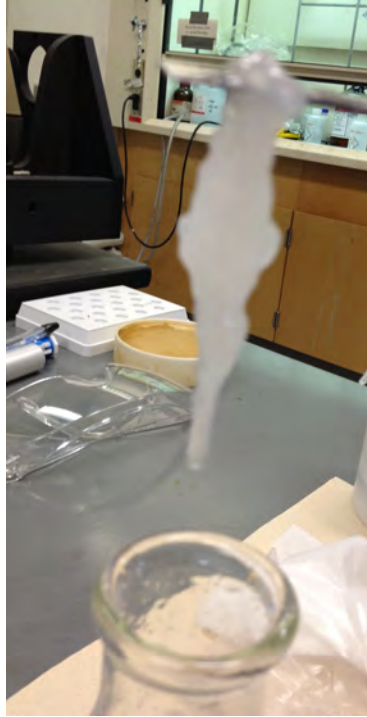
Figure 2.5 Hydrogel material system comprised of cellulose nanowhiskers and collagen forming the COL-CNW composite upon magnetic stirring.
