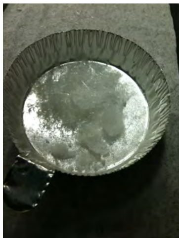
Figure 2.2 Freeze-dried cellulose nanowhiskers directly from the freeze-dryer and measured by weight prior to mixing with the biopolymer matrix and forming the nanocomposites of CAP-CNW and COL-CNW.
