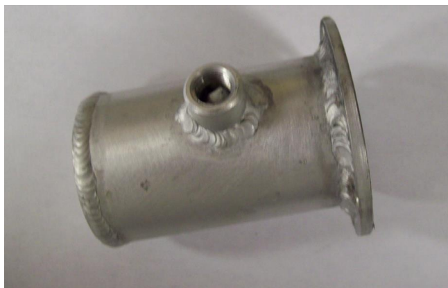
Figure 5.5 Bed #2, Aluminum, larger capacity, lower thermal mass
