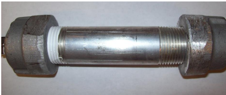
Figure 5.8 Bed #3 without the external fins attached. This bed damaged by a faulty heater.
