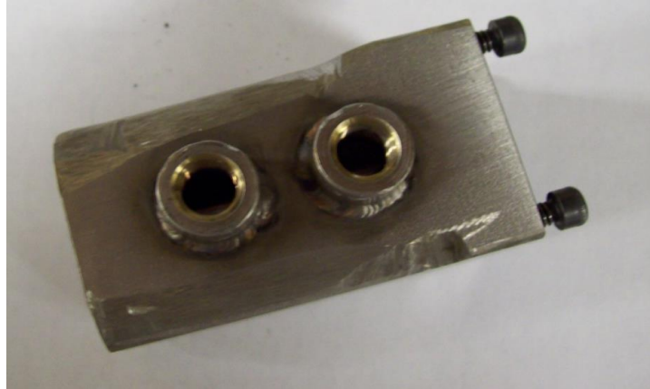
Figure 5.3 Bed #1 constructed of stainless steel.
