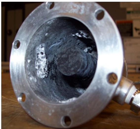
Figure 5.6 Corrosion within the bed due to contamination of ammonia with water
