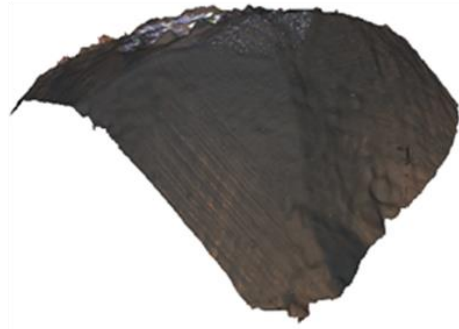
(a) Initial diamond dresser geometry
