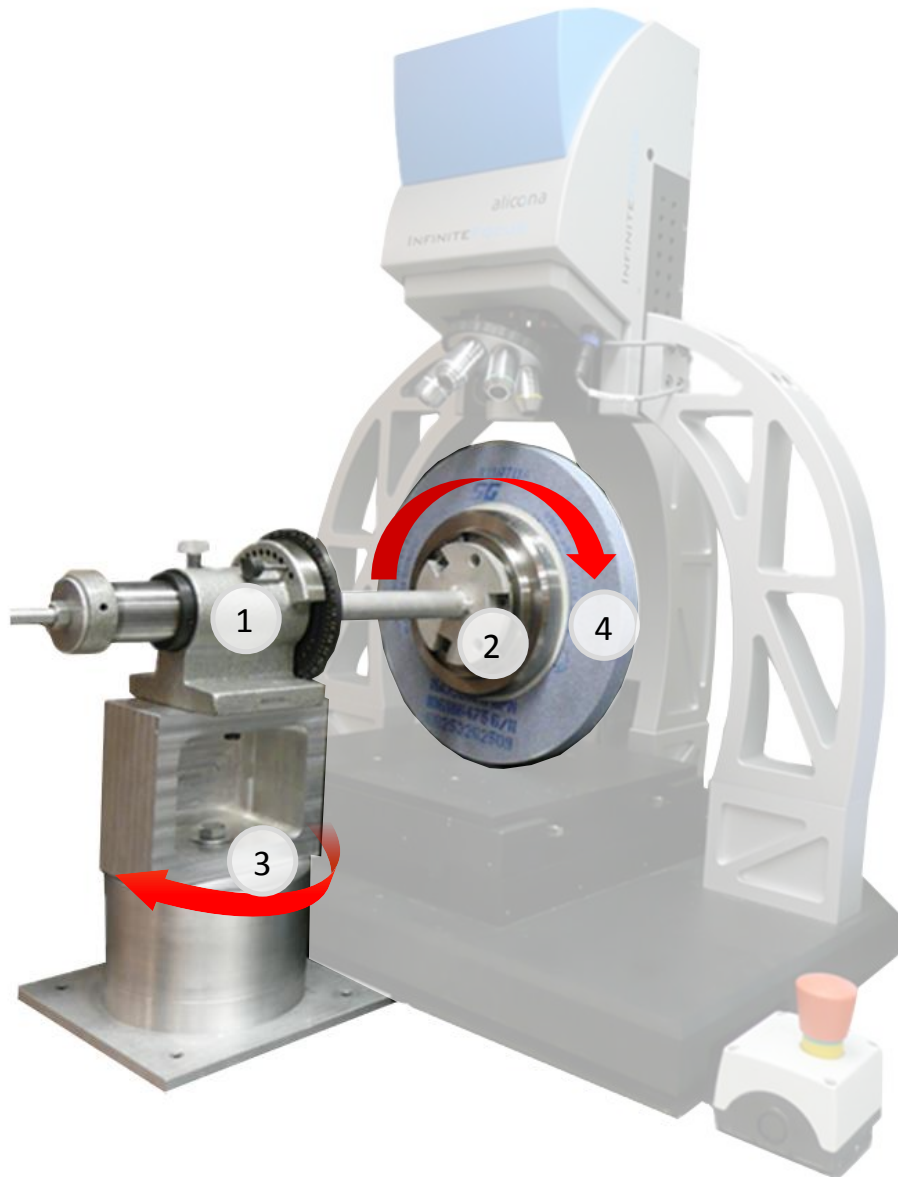
Figure 4.11 – Precision indexing apparatus to align grinding wheel for pre- and post- grinding measurements. (1) indexing head, (2) precision hub adapter/locator, (3) base pivot for loading/unloading wheel, and (4) grinding wheel
