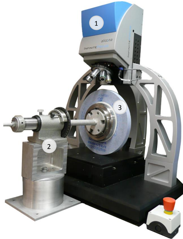
Figure 4.2 – Experimental setup used to measure grinding wheel surface topography. (1) optical surface measuring instrument, (2) wheel indexer, (3) grinding wheel
