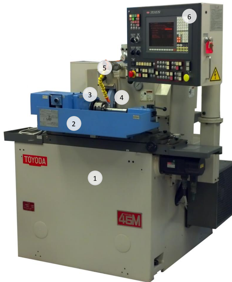
Figure 4.5 – Precision grinding machine. (1) machine base, (2) workpiece slide table with work head, (3) dresser mounted on back of slide table, (4) grinding wheel, (5) coolant nozzle, (6) controller of grinding machine
