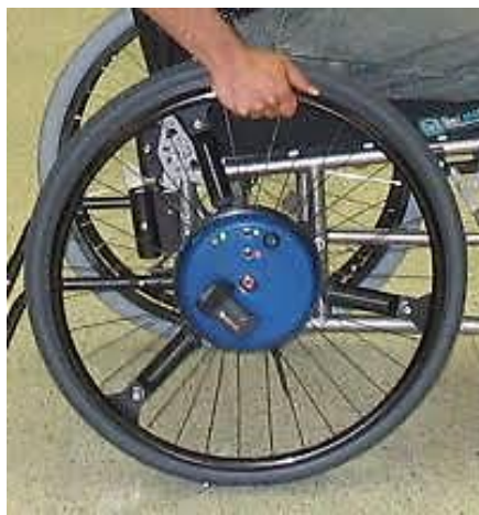
Figure D.6 Rolling resistance test using an instrumented wheelchair.
