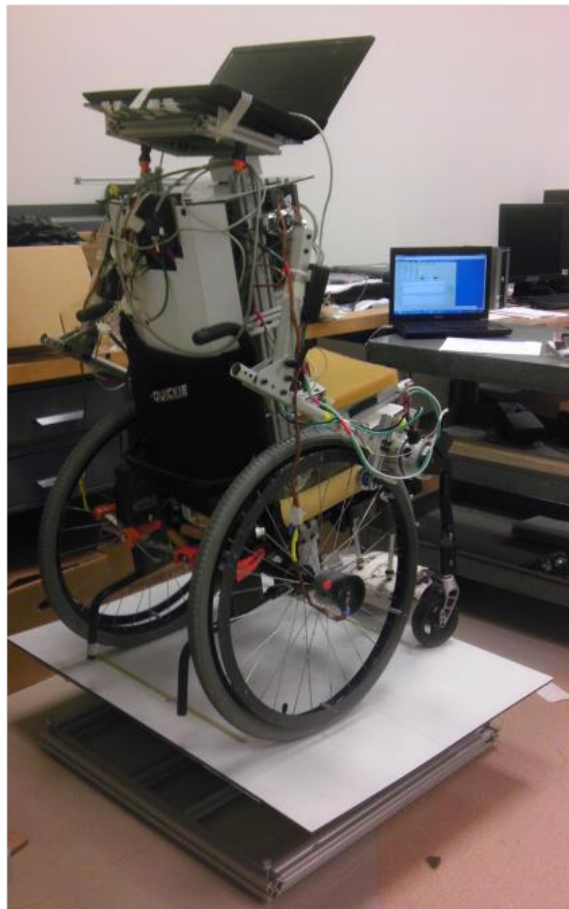
Figure 3.4 Pendulum platform used measure AMPS inertial properties
