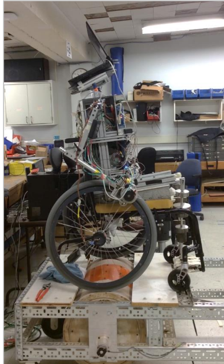
Figure 6.36 AMPS on a single-roller dynamometer.
