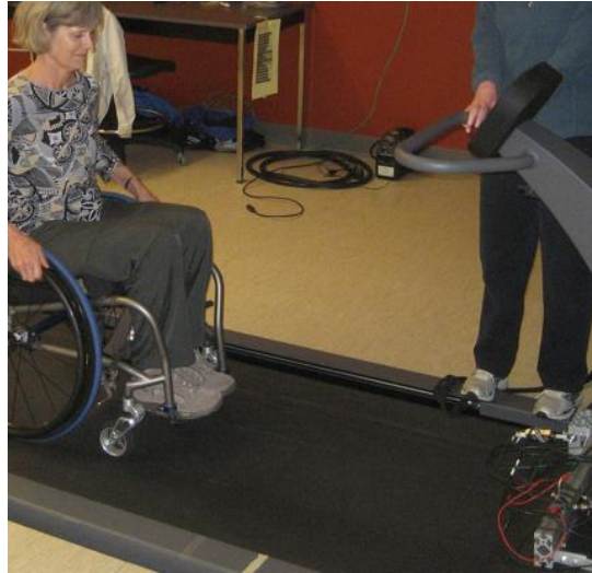
Figure D.5 Rolling resistance test using a treadmill.
