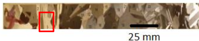
Figure 5-5: NIR transmission image of a multicrystalline beam, bright grain highlighted.
