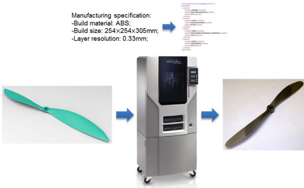
Figure 3-14 Build the propeller of the drone using 3D printing [171]
