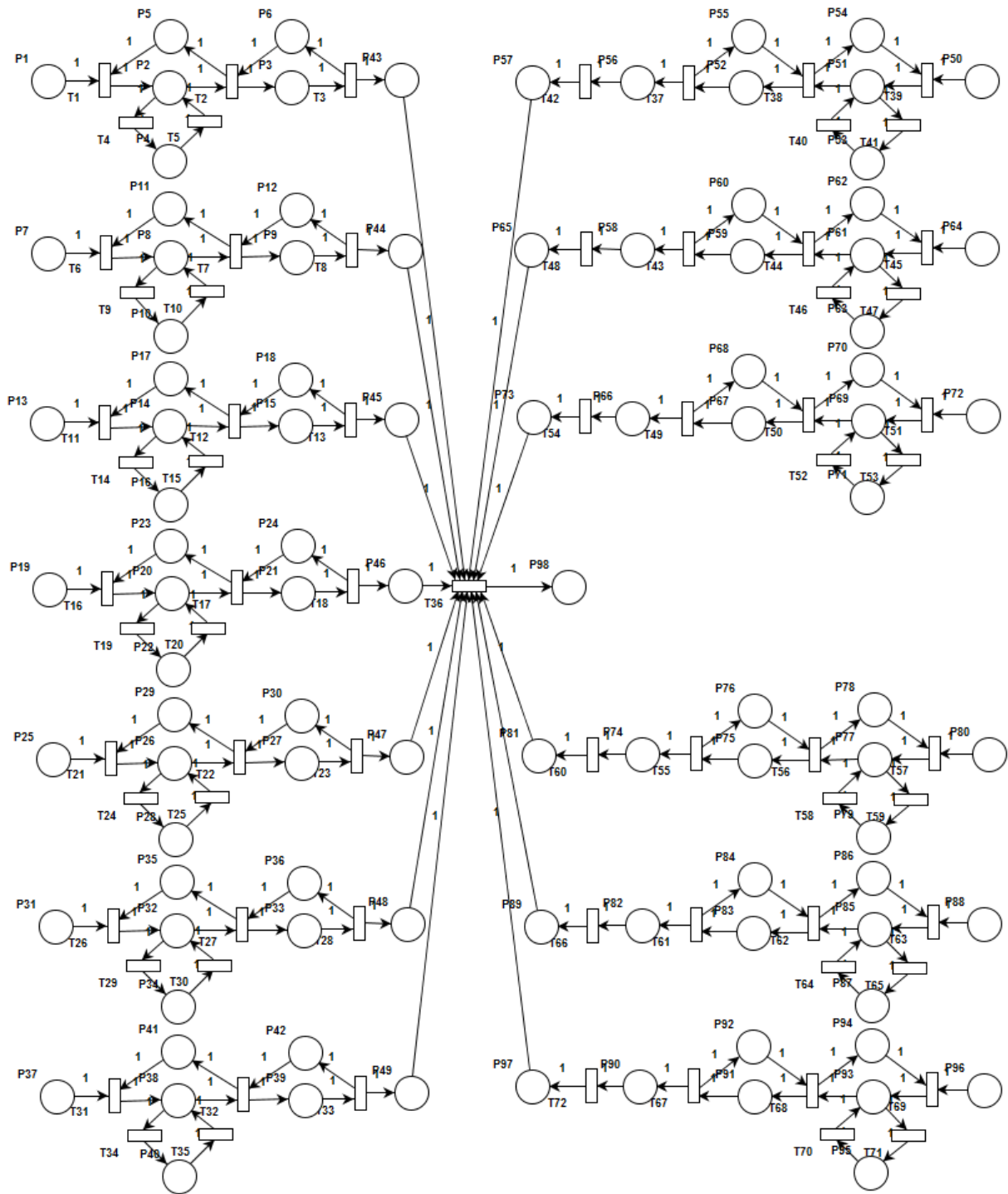
Figure 6-16 SPN for modeling the entire manufacturing system
