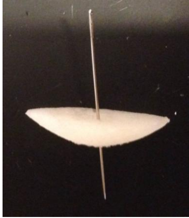
Figure 18: Method to Create Poked Holes in PVA
