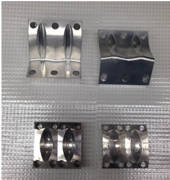
Figure 8: Aluminum Molds of for Chin and Nasal Implant
