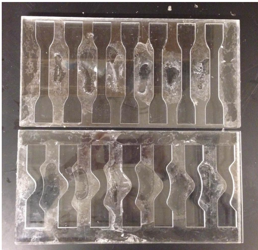
Figure 12: Acrylic Molds Used to Create Samples for Tensile Tests
