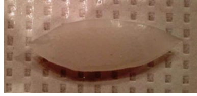
Figure 21: 30% wt PVA Molded over Velcro
