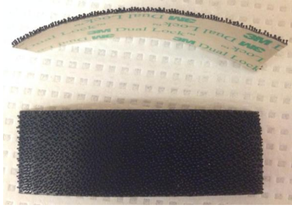
Figure 17: Velcro Used to Mold Pores in PVA cryogel
