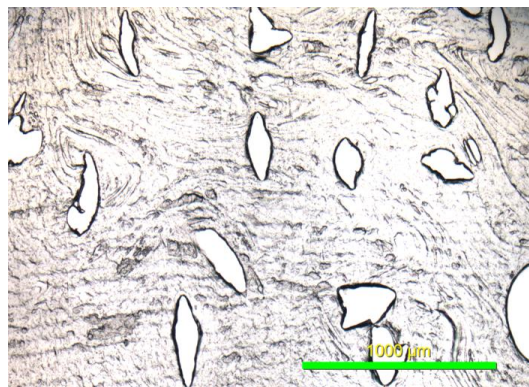
Figure 34: Sectioned Images of 30% wt PVA cryogel pressed with a 500 \mu\text{m} needle
