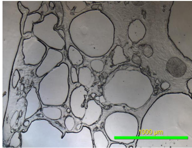
Figure 37: Sectioned Image of Porous PVA cryogel Created Through Gas Method
