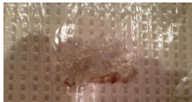
Figure 23: Porous PVA Cryogel Created through Gas Method with 20% wt PVA cryogel
