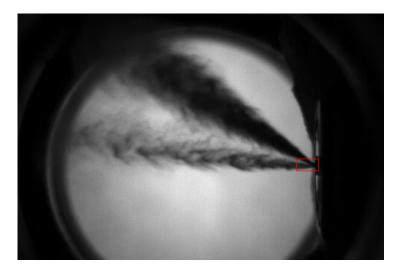
Figure 33: Shadowgraph of the whole spray at atmospheric temperature and pressure and 3000 psi injection pressure
