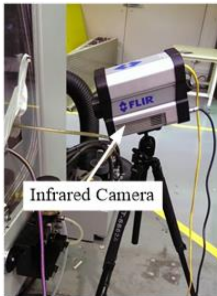
Figure 6.7 Infrared camera set-up
