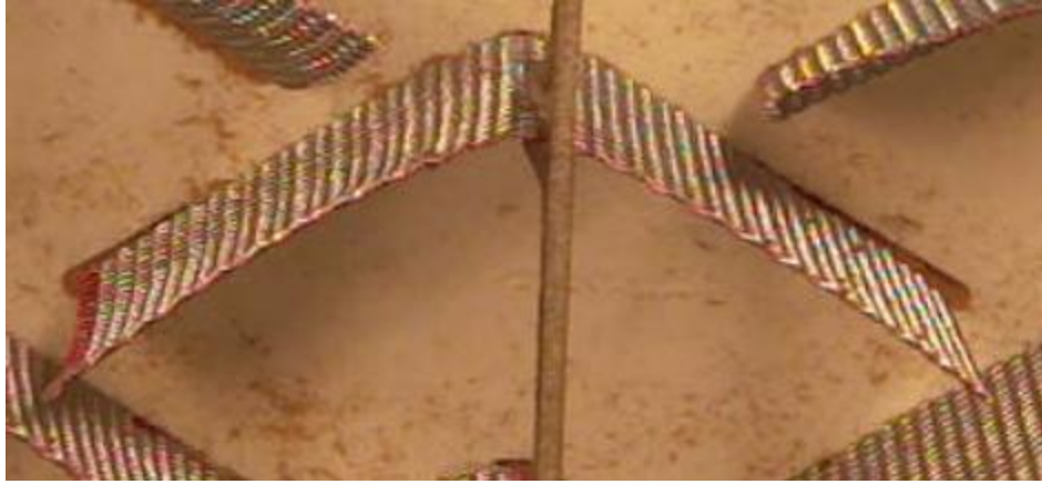
Figure 1.2 Discrete Porous Structure Wire Mesh Chevron Configuration
