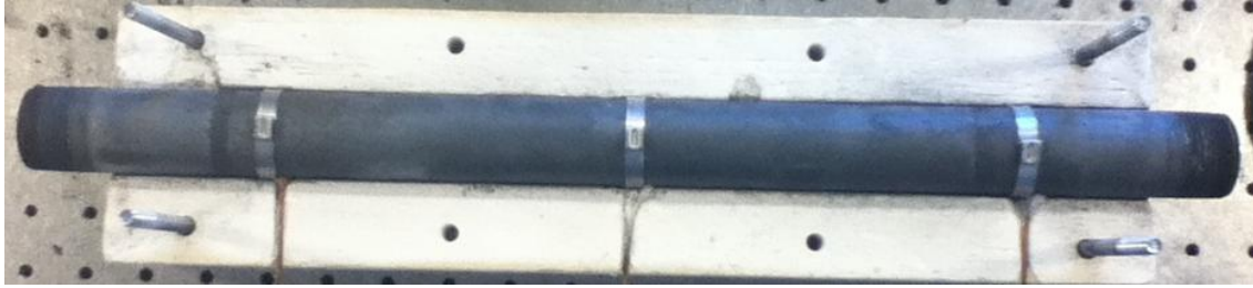
Figure 3.5 SS316 Pipe Sitting in Duraboard Insulation Fitted to Pipe with External K-Type Thermocouples Fixed in Place
