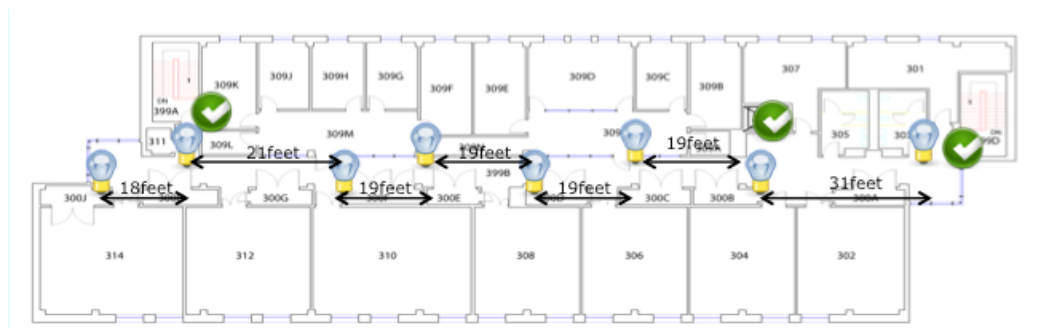
Figure 51 Deploy layout in Knowles Engineering building
