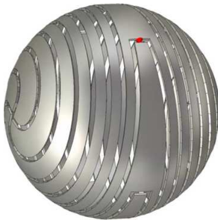
Figure 6.1. Depiction of a 4-arm folded slot spherical helix magnetic dipole [16].
