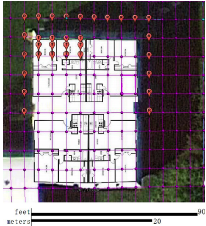
Figure 3.4: Experimental area: 'R' points represent RPs, 'T' points represent TPs.
