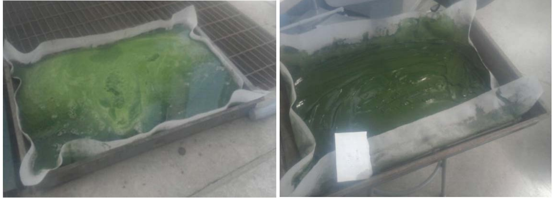
Figure 2.19: Left: Algae slurry after decantation; ~2 wt% Right: Algae paste after gravity drainage; 13 wt%.
