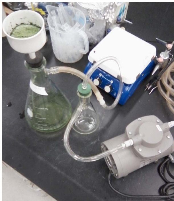
Figure 2.21: A vacuum pump attached to a filter flask with a Buchner funnel. House vacuum can also be attached.
