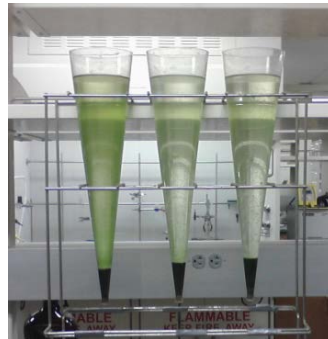
Figure 3.2: Imhoff settling cones used for triplicate sedimentation testing displaying a liquid supernatant layer above and slurry layer containing solids below.
