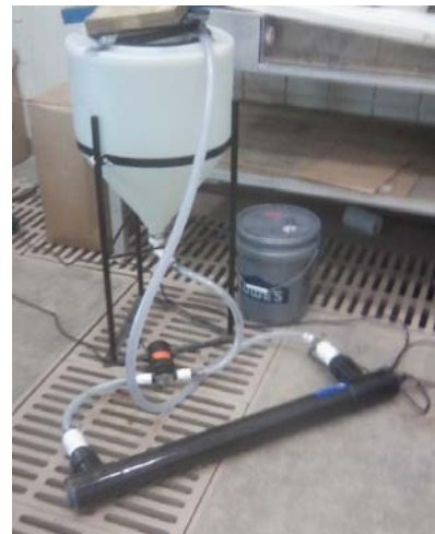
Figure 2.18: Harvesting process. Top-Left: Suspending flocculant in a solution. Top-Right: The flocculant is mixed in a harvest tank. Bottom-Left: Algal slurry is applied to in-house belt filter. Bottom-Right: Make-up supernatant water with UV Sterilizer.
