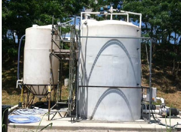
Figure 2.23: East Bend Reactor. Left: Harvest tank, 6,000 L. Right: Process tank, 15,000 L.
