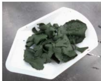
Figure 2.22: Cake solids produced from vacuum filtration; 20-25 wt%.
