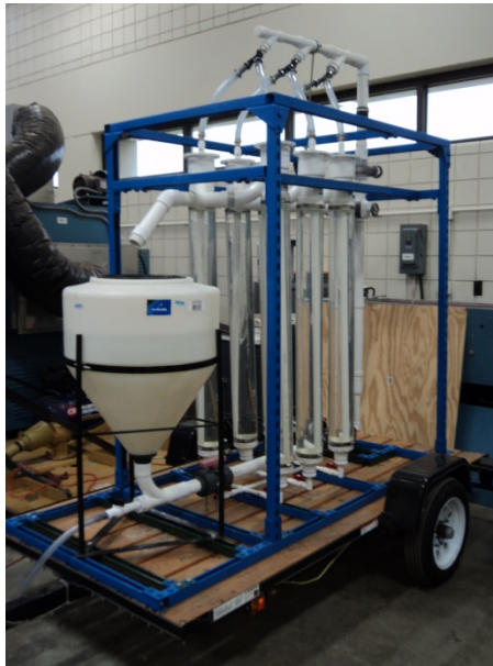
Figure 2.16: Trailer reactor located indoors at BAE; 115 L.
