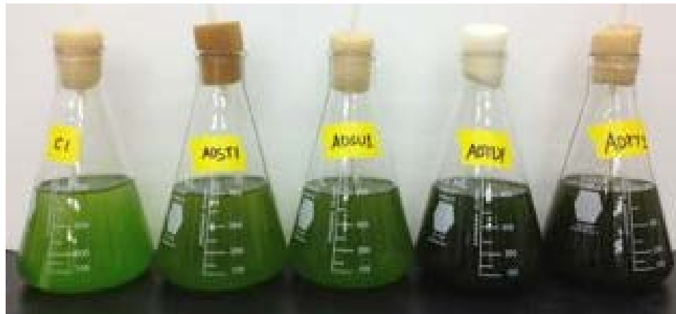
Figure 5.8 The effect of liquid and solid digestate on culture color and turbidity. From left to right, flasks contain fresh urea media, tap water mixed with liquid digestate, fresh urea media mixed with liquid digestate, tap water mixed with total digestate and fresh urea media mixed with total digestate.
