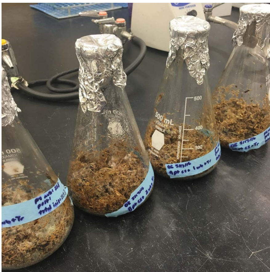
Photo line-up of samples with 7, 8, 9, and 10 g pretreated corn stover and 3, 2, 1, and 0 g of wheat bran (left to right) after seven days of incubation. Notice the apparent difference in colonization by T. reesei RUT-C30 between the far left sample and the far right.
