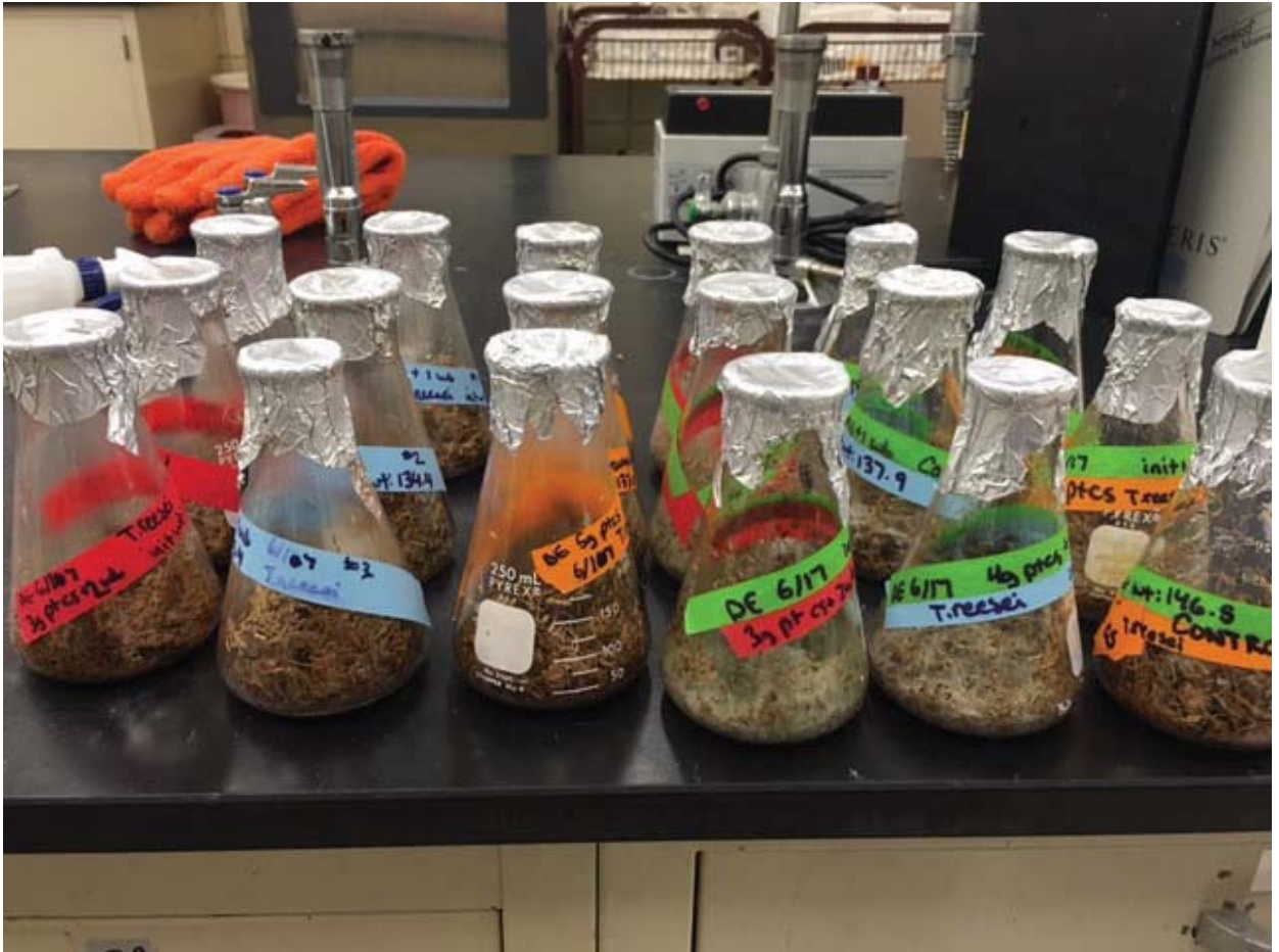
Picture of samples after SSC and hydrolysis in Objective II. From samples on the left side of the picture were stored at 50°C for five days after seven days of storage at 30°C. From left to right, the samples contain three grams of corn stover and two grams of wheat bran; four grams of corn stover and one gram of wheat bran; and five grams of corn stover. Samples on the right side of the picture were stored at 30°C for 12 d and from left to right contain three grams of corn stover and two grams of wheat bran; four grams of corn stover and one gram of wheat bran; and five grams of corn stover. All corn stover was pretreated with 0.1 N sodium hydroxide for two hours at room temperature.
