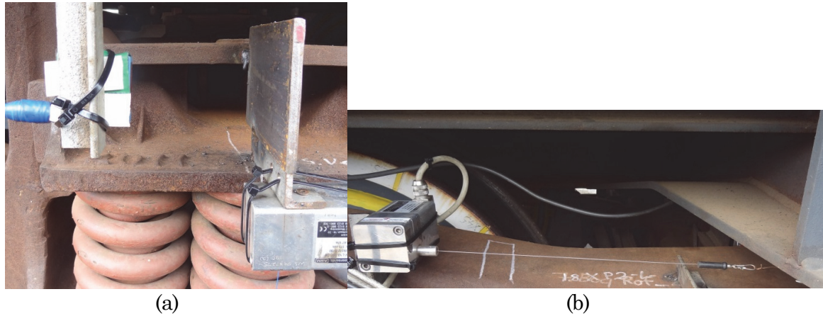
Figure 2-7: Measurement of bogie rotation relative to the wagon body (a) with a laser and (b) with a rope displacement transducer
