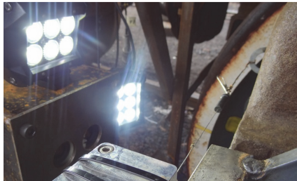
Figure 2-10: Stereo vision cameras mount to measure primary suspension displacements
