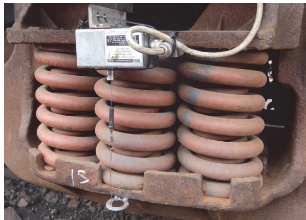
Figure 2-6: Measurement of secondary suspension displacement
