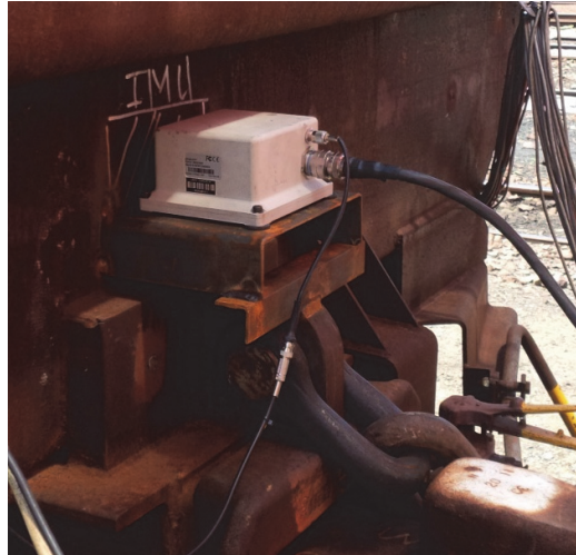
Figure 2-12: Location of the IMU measuring body responses
