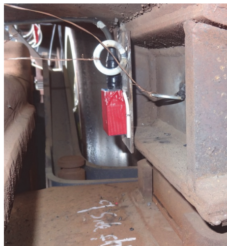
Figure 2-11: Measurement of body displacement relative to the bolster
