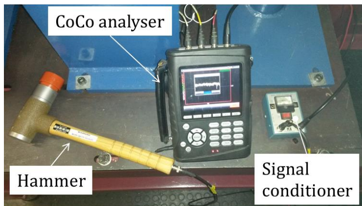
Figure G-3: Modal impact hammer, CoCo FFT analyser and signal conditioner used in dynamics measurements of the setup test-bench
