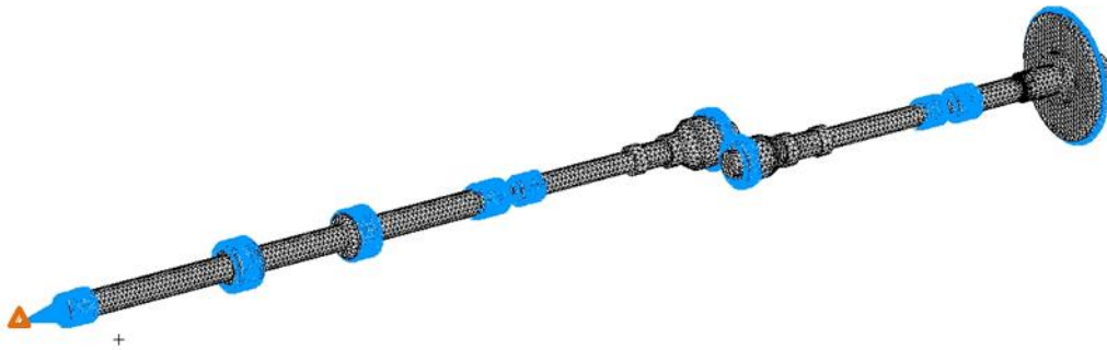
Figure 3-5: Multipoint constraints on the mesh of the drivetrain.
